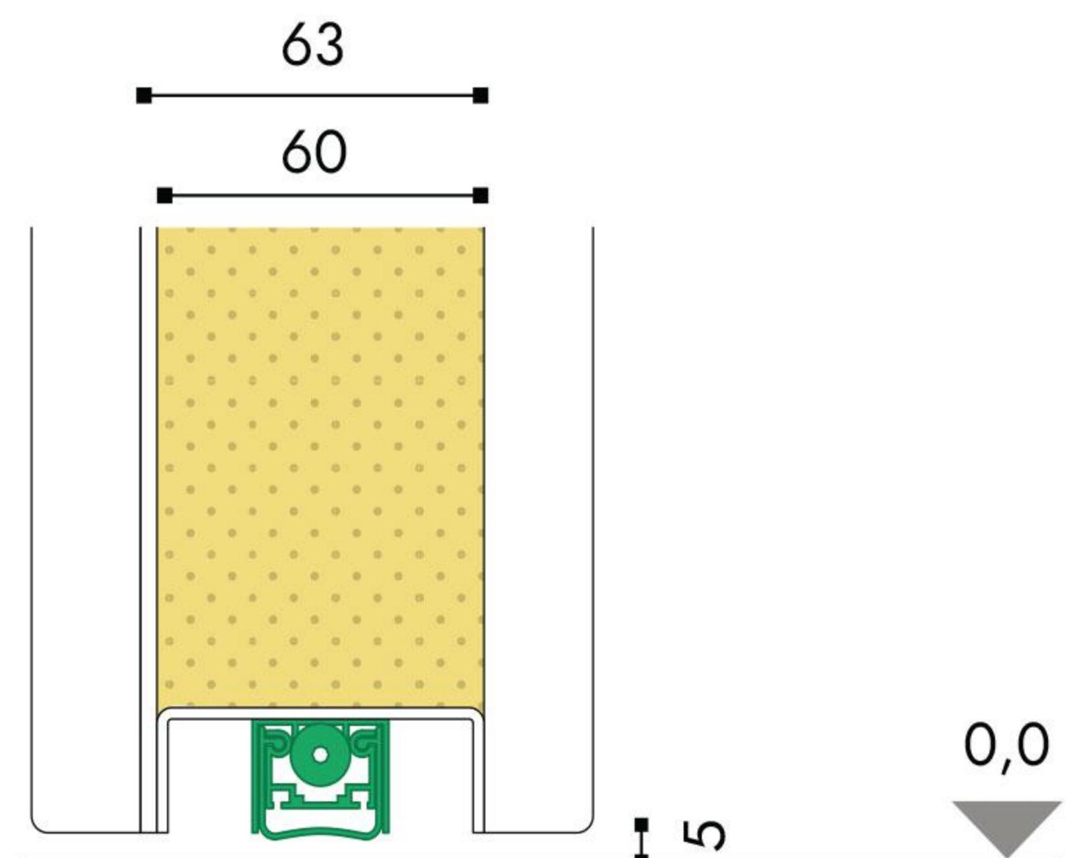
FOR EXTERNAL USE
